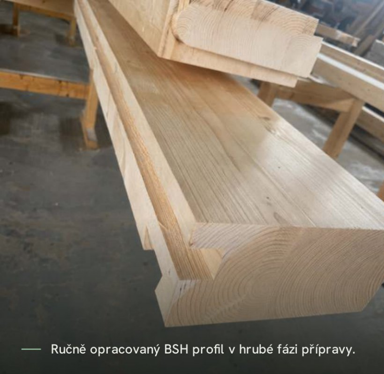
— Detail BSH hranolu — slepené a sušené lamely.
