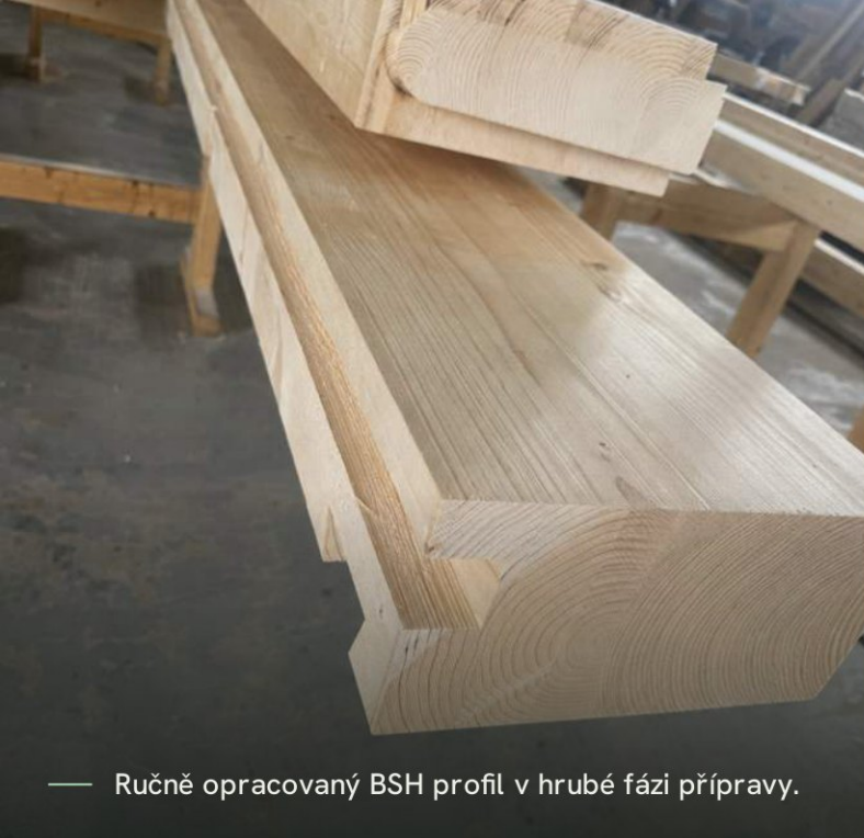
— Detail BSH hranolu — slepené a sušené lamely.
